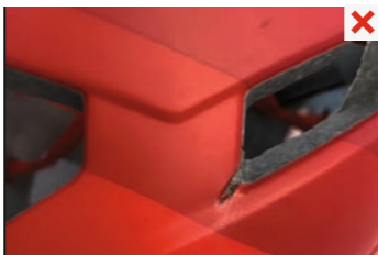
damaged helmet absorber
