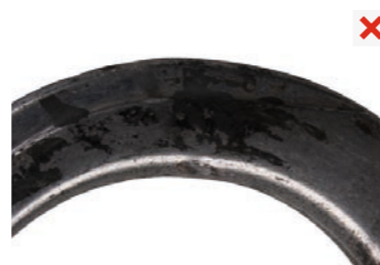
lock failure and damaged part
