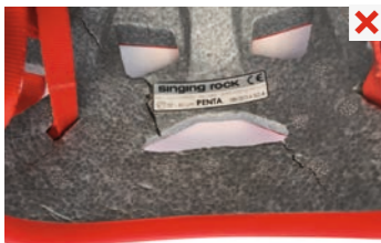
broken construction of the helmet absorber
