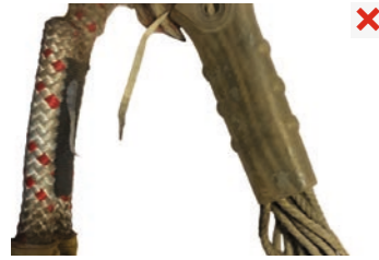
damaged sheath and core
