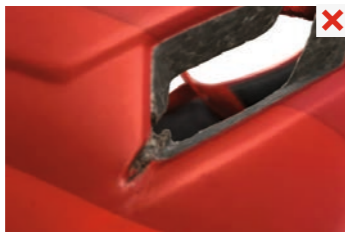
damaged adjustment system
