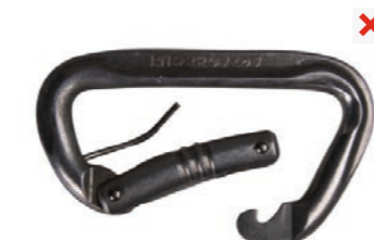
broken swinging hinge
